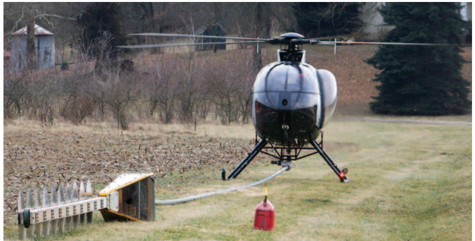
Helicopter is ready to take saw array to the air.
